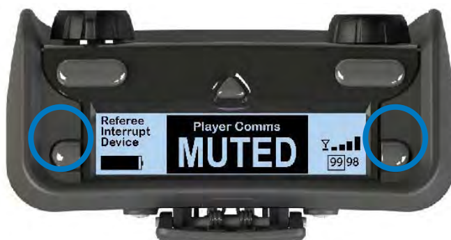
Figure 124: Referee Radio Pack Function Buttons
