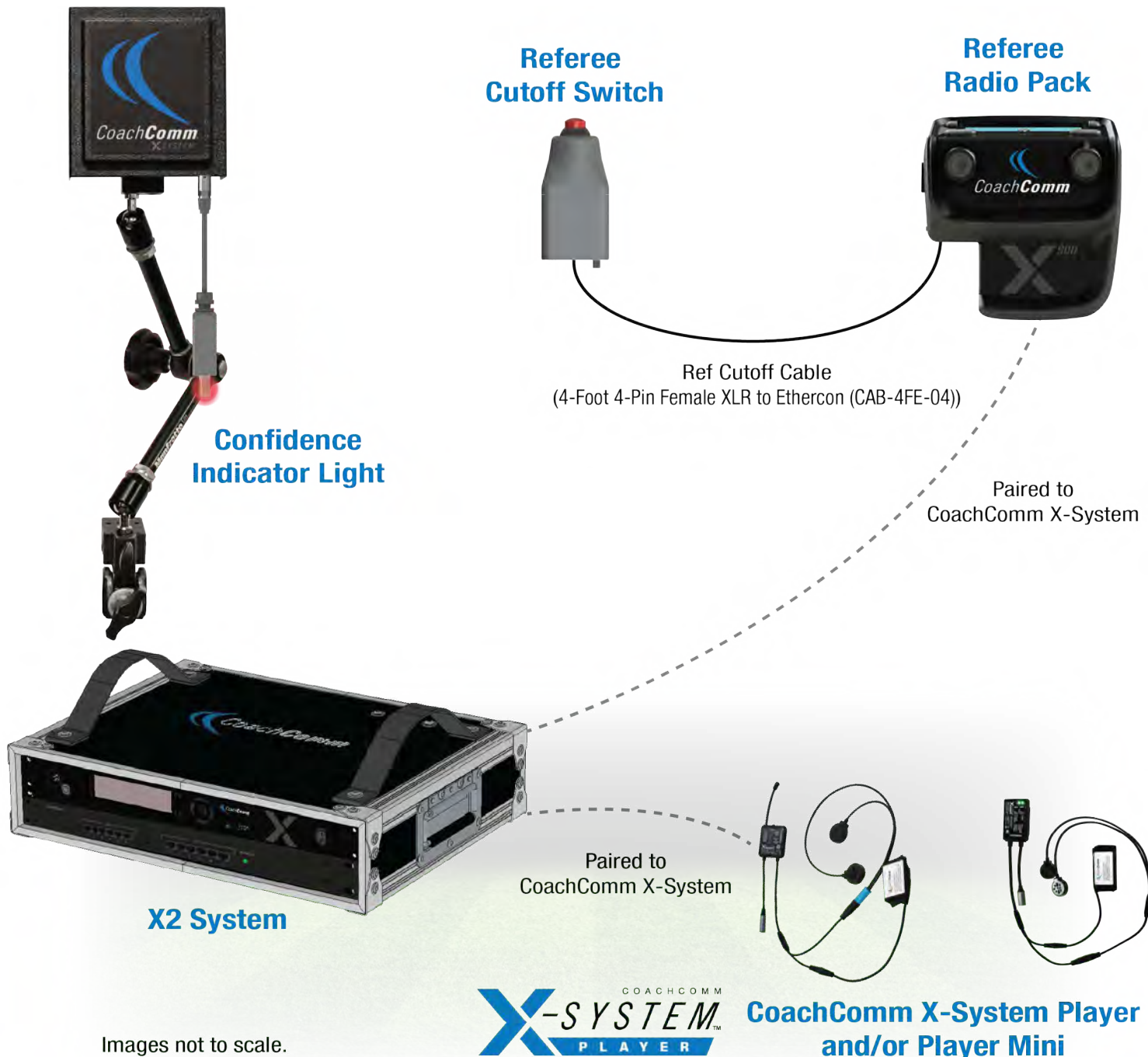
Figure 109: CoachComm X-System Player Block Diagram (Single Wirelless Referee Interrupt Configuration)
