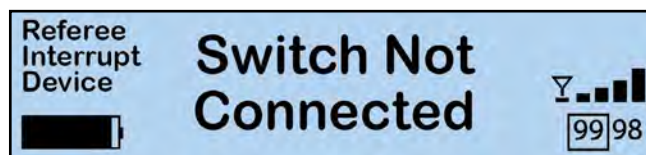
Figure 118: Referee Radio Pack Switch Not Connected
