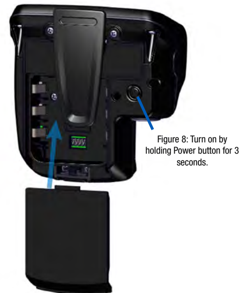
Figure 9: RP Battery Installation and Power On
