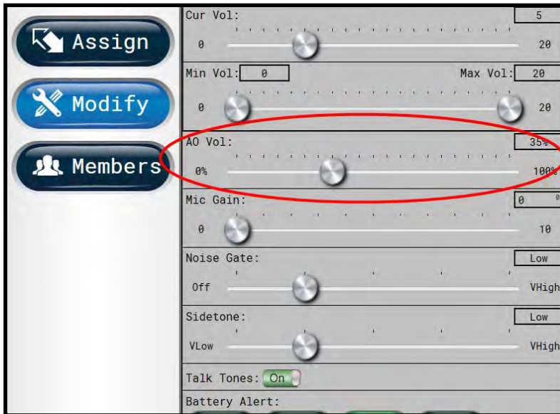
Figure 94: AO Volume Setting on Profile Screen
