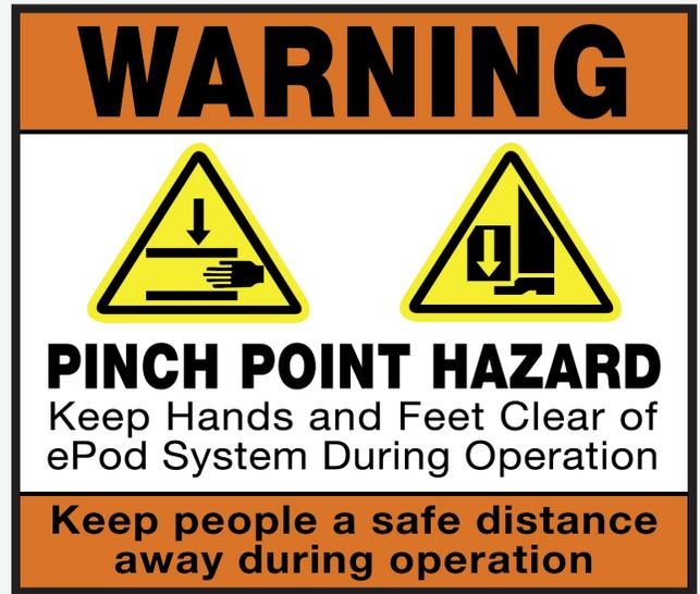
Figure 4: This warning label is attached to each ePod and alerts users of specific pinch hazards.
