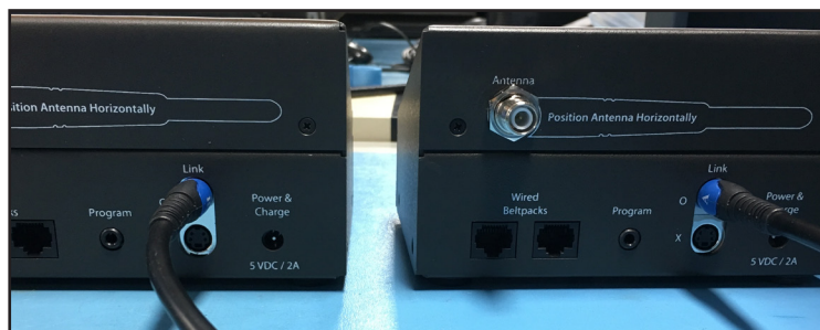
Sample Link Cable Connection Between O Ports. During normal operation, the Command Centers should be positioned farther apart than shown here.
