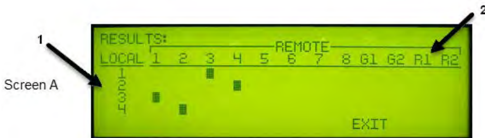
Figure 33: WIM 8 Dry Pair Testing Fault Screen
