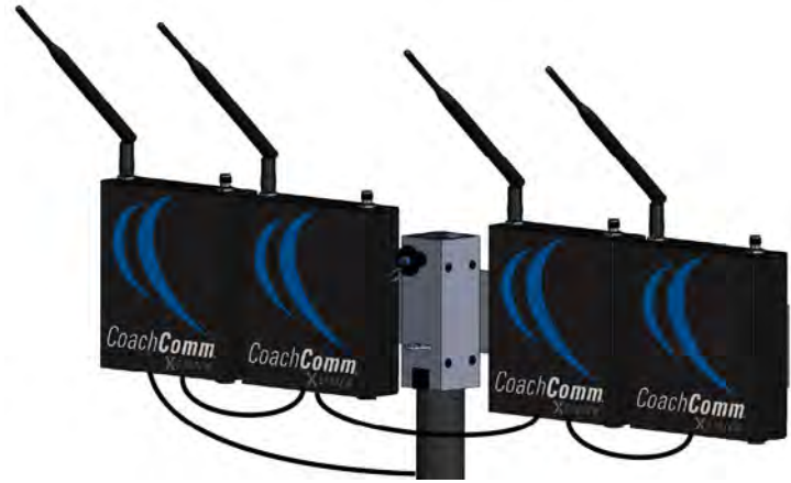
Figure 112: One Sideline Trunk RT Mounting Bracket on the RT Mast (Cables Not Shown)
