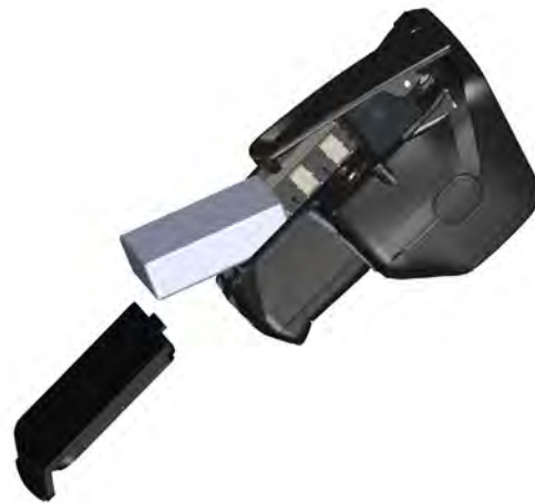
Figure 48: Radio Pack Battery Installation
