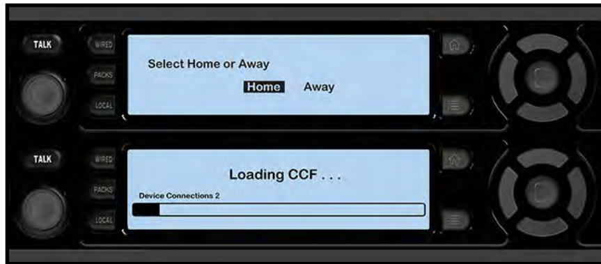
Figure 59: CU Home/Away Prompt and Progress Bar
