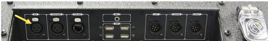
Figure 14: I/O Connection Panel Mic Connection
