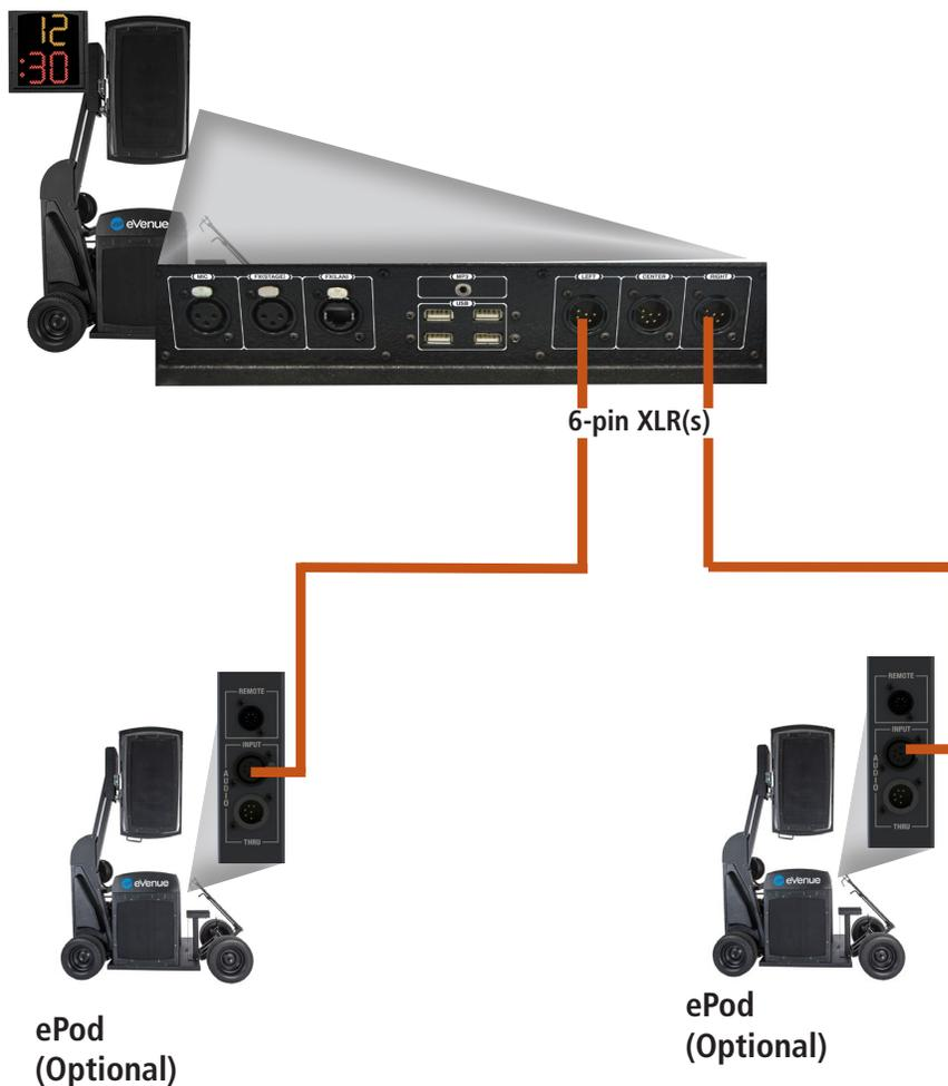
Figure 9: eVenue Tempo Audio Cable (from rear of Control Unit) to additional optional ePods
