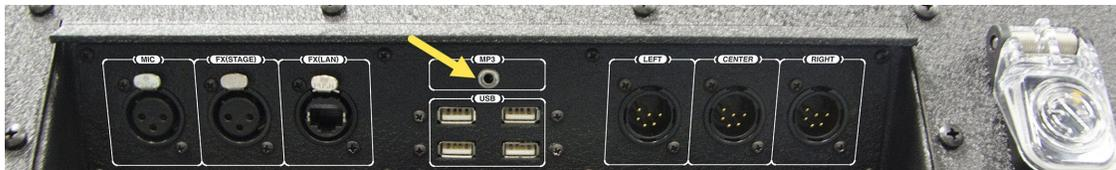
Figure 17: Tempo Control Unit MP3 Port
