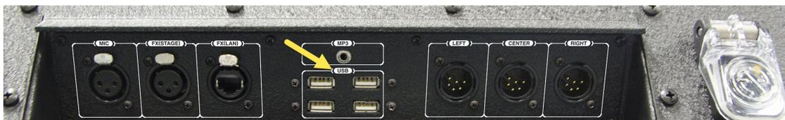
Figure 19: Tempo Control Unit USB Ports
