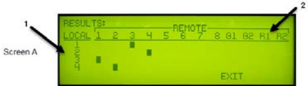
Figure 32: WIM 8 Dry Pair Testing Fault Screen
