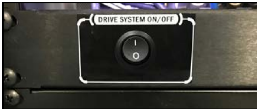
Figure 26: Drive System Switch (On Position)
