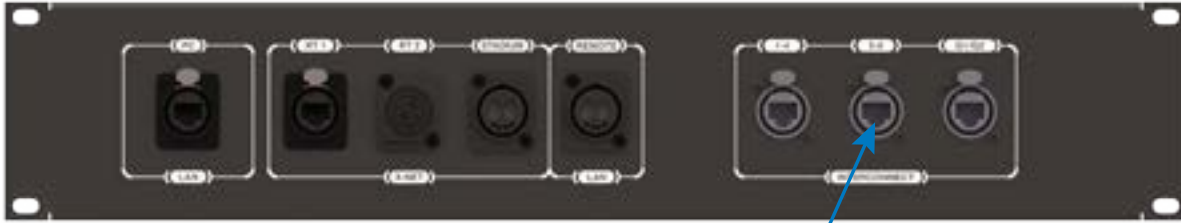
Wireless Press Box Unit (WPB2) Rear Panel
