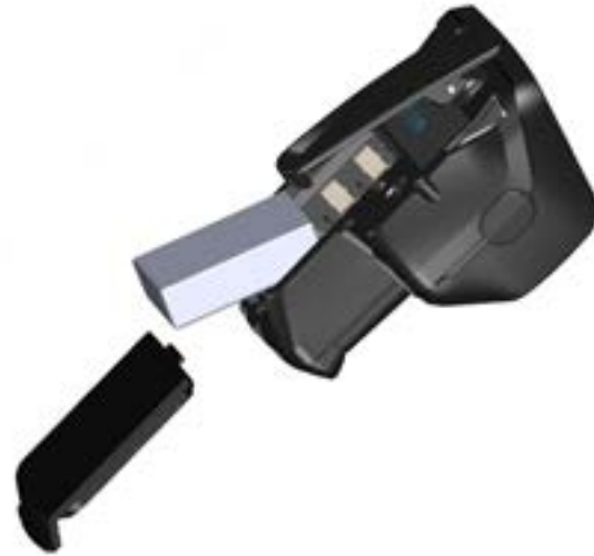
Figure 31: Radio Pack Battery Installation
