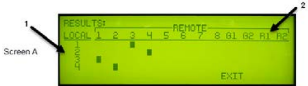
Figure 24: WIM 8 Dry Pair Testing Fault Screen
