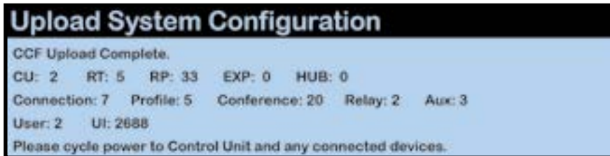
Figure 55: CU LCD: Sample CCF Upload Completed Screen
