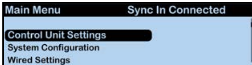
Figure 101: Sync In Indicator on CU Primary Operating Screen
