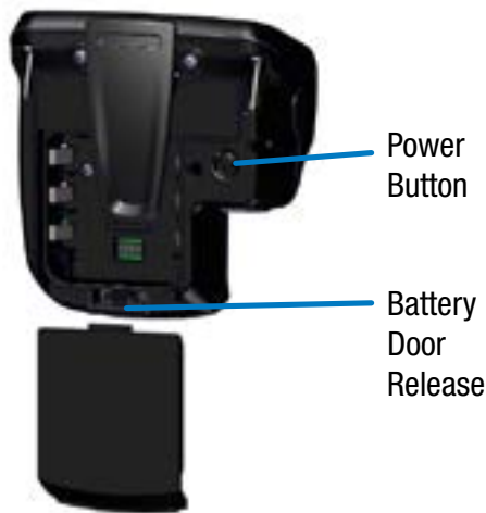
Figure 44: Rear View of RP's Power Button and Battery Door
