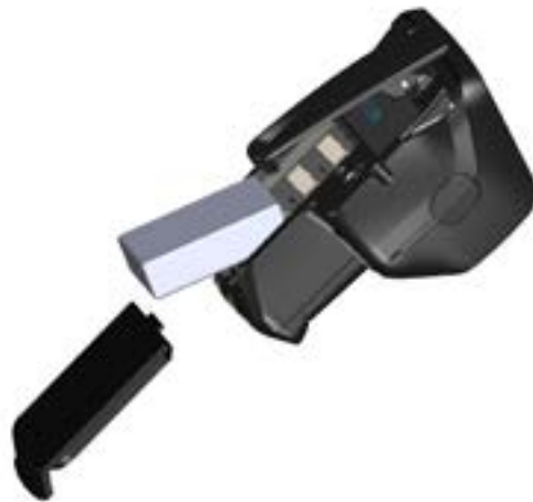
Figure 45: Radio Pack Battery Installation
